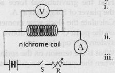
What is the reading for not showing any deflection by the voltmeter and ammeter even though the switch 'S' its closed?
